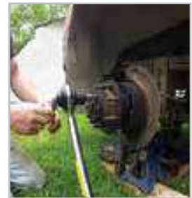
Torque multiplier used for lug nuts
