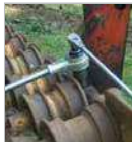
Torque multiplier used on tracks
