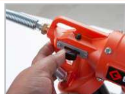
Slide backwards for Continuous Mode
