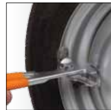
Hammer end being used to form wheel balancing weights
