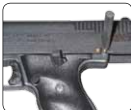
Roll Pin Punch being used to remove spring pin from a gun
