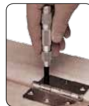
Punch being used to mark screw starting centres on a door frame
