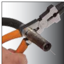
Nozzle removal & installation
