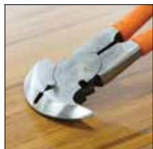
Main jaw for pulling out nails
