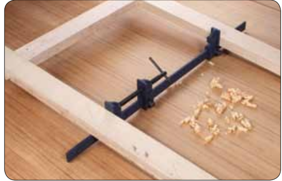
Duo Bar used for internal clamping
