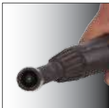
Welding Gun Nozzle filled with weld spatter
