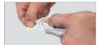
When blunt, simply pull out blade, invert it & re-install
